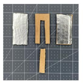
**Step 5:** Take the piece of card that you removed from the centre rectangle and cut a V shape out of the top to make it easier to place it inside your switch.
