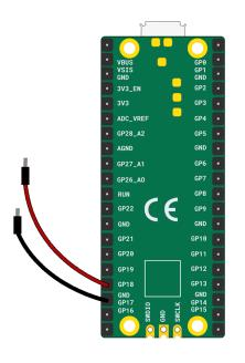
**Tip:** When you craft a switch you will stick the pin end of the jumper wire to a conductive surface, like copper taper or kitchen foil.
