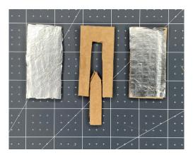
**Step 7:** Cover the removed piece in **aluminium foil**. It is very important that you use one piece of foil and that it wraps all the way around. This is what will make the switch close and allow the current to flow.
