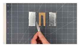
**Step 8:** Next, use some sticky tape to secure the pin end of two jumper wires to the top of each rectangle. It is important that the pins make a secure contact with the aluminium foil. Make sure that each pin is lying flat against the foil with the plastic part of the jumper wire against the edge of the cardboard.
