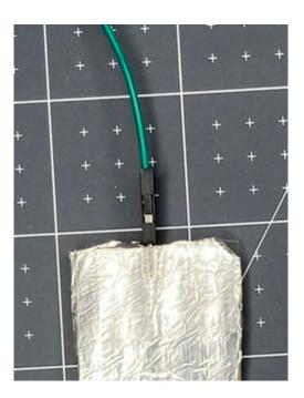
Step 9: Add more tape to secure the jumper wire and stop it from accidentally coming loose.
