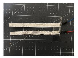
**Step 3**: Stick some kitchen foil or conductive tape to the bottom of an object. The base must be large enough to create a connection between the two wires.
