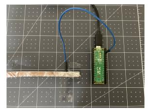
**Step 3**: When adding a component to the Raspberry Pi Pico, connect the **positive** end to a **GP** pin and the **negative** end to the kitchen foil.
