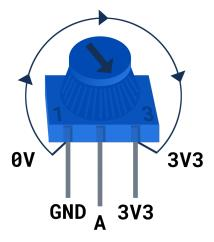
**Connect:** Find three socket-socket jumper wires and attach one to each leg of the potentiometer. You may wish to secure the legs with some electrical tape if they feel loose.
