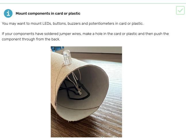
If you are using components with socket-socket jumper wires then remove the jumper wires and push the legs of the component through card. For plastic you will need make holes first by carefully using a tool with a sharp point.
