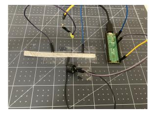
**Step 4**: When adding further components, ensure that the **positive** end is connected to a **GP** pin on the Raspberry Pi Pico and that the **negative** end is stuck to the kitchen foil.
